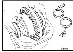
14. Insert selected left and right side bearing adjusting washers in place between side bearings and gear carrier. Refer to <a href="DLN-98">DLN-98</a>. <a href="mailto:">"M/T : Adjustment"</a>.
