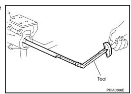
Place the J-34309-11 "R200A" pinion height adapter onto the gauge plate and tighten it by hand.
