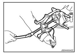
5. Press drive pinion assembly out of gear carrier.
