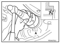
3. Align the matching mark (B) of drive pinion with the matching mark (A) of companion flange (1), and then install the companion flange (1).
