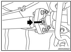
Loosen mounting nuts of center bearing mounting brackets.CAUTION:
