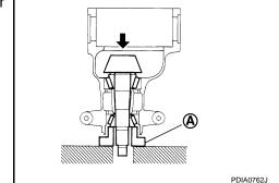
8. Using the drift (A) [SST: ST30720000 (J-25405)], install front oil seal as shown in figure.
