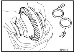
4. Insert left and right original side bearing adjusting washers in place between side bearings and gear carrier.
