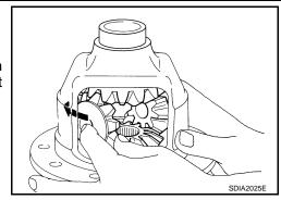
5. Align the lock pin holes on differential case with shaft, and install pinion mate shaft.
