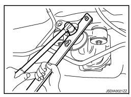
11. Remove companion flange using pullers.
