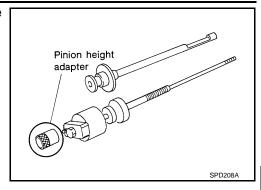
8. Position the side bearing discs, J-25269-4, and arbor firmly into the side bearing bores. Install the bearing caps and tighten bearing cap mounting bolts to the specified torque. Refer to <a href="DLN-91">DLN-91</a>. <a href="mailto:"M/T : Exploded View"</a>.
