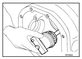
4. Assemble the pinion front bearing inner race and the J-34309-2 gauge anvil. Assemble them together with the J-34309-1 gauge screw in gear carrier. Make sure that the pinion height gauge plate, J-34309-16, turns a full 360 degrees. Tighten the two sections together by hand.
