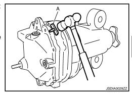
Using two 45 mm (1.77 in) spacers, mount carrier on the attachment (A) [SST: KV38100800 (J-25604-01)].
