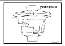
14. Loosen screws on differential cases A and B.
