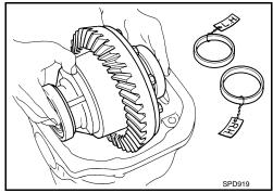
Remove side bearing inner race.
