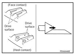
• If the tooth contact is near the flank (flank contact), or near the toe (toe contact), thin pinion height adjusting washers to move drive pinion farther from drive gear.
