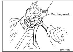
Loosen mounting nuts of center bearing mounting brackets.
