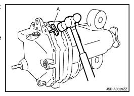
5. Using two 45 mm (1.77 in) spacers, mount carrier on the attachment (A) [SST: KV38100800 (J-25604-01)].
