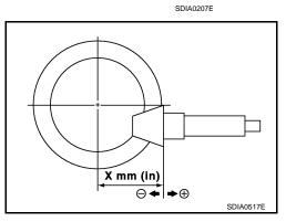
• If the tooth contact is near the face (face contact), or near the heel (heel contact), thicken pinion height adjusting washers to move drive pinion closer to drive gear.
