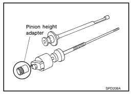
Position the side bearing discs, J-25269-4, and arbor firmly into the side bearing bores. Install the bearing caps and tighten bearing cap mounting bolts to the specified torque. Refer to <u>DLN-103</u>, "A/T: Exploded View".
