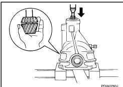
10. Remove pinion rear bearing inner race and pinion height adjusting washer with the replacer (A).
