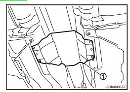
5. Put matching marks on propeller shaft rubber coupling with final drive companion flange.
