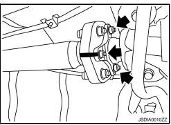
8. Slightly separate the rubber coupling (1) from the final drive companion flange (2).
