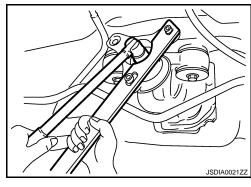
11. Remove companion flange using pullers.
