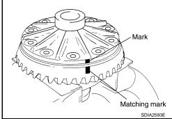
9. Apply thread locking sealant into the thread hole of drive gear.
