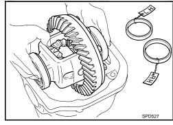
14. Insert selected left and right side bearing adjusting washers in place between side bearings and gear carrier. Refer to <u>DLN-45</u>. "Adjustment".
