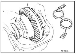
9. Remove side bearing inner race.
