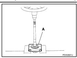
11. Tap pinion front/rear bearing outer races uniformly using a brass rod or equivalent to remove them.
