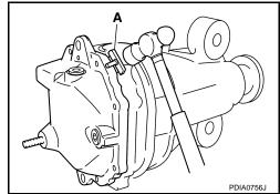
Using two 45 mm (1.77 in) spacers, mount carrier on the attachment (A) [SST: KV38100800 (J-25604-01)].
