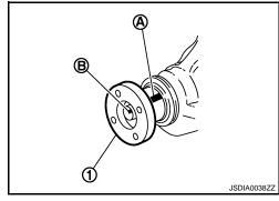
10. Remove drive pinion lock nut using the flange wrench.
