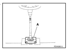
11. Tap pinion front/rear bearing outer races uniformly using a brass rod or equivalent to remove them.
