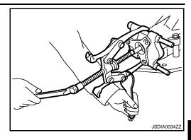
Press drive pinion assembly out of gear carrier. CAUTION:
