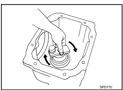
6. Measure the turning torque at the end of the J-34309-2 gauge anvil using preload gauge [SST: ST3127S000 (J-25765-A)].
