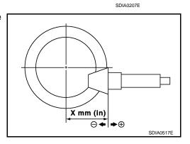
• If the tooth contact is near the face (face contact), or near the heel (heel contact), thicken pinion height adjusting washers to move drive pinion closer to drive gear.
