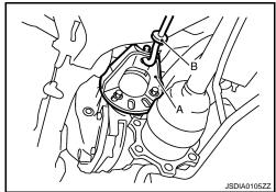
Remove side oil seal, using a flat-bladed screwdriver. CAUTION:
