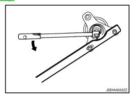
3. Put matching mark (B) on the end of drive pinion. The matching mark should be in line with the matching mark (A) on companion flange (1).
