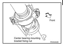
Remove propeller shaft assembly fixing bolts and nuts.
