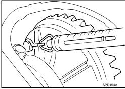
8. If the turning torque is outside the specification, use a thicker/thinner side bearing adjusting washer to adjust.
