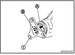
10. Apply anti-corrosion oil to the thread and seat of drive pinion lock nut, and temporarily tighten drive pinion lock nut to drive pinion.
