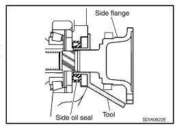
Put a suitable drift on the center of side flange, then drive it until sound changes.
