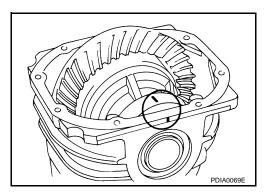
17. Using the drift [SST: KV38100200 (J-26233)], drive side oil seals until it becomes flush with the case end.
