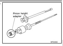
8. Position the side bearing discs, J-25269-4, and arbor firmly into the side bearing bores. Install the bearing caps and tighten bearing cap mounting bolts to the specified torque. Refer to <a href="DLN-51">DLN-51</a>. <a href="Exploded View"</a>.
