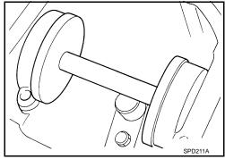
Select the correct standard pinion height adjusting washer thickness. Select by using a standard gauge of 3 mm (0.12 in) and J-34309-101 feeler gauge. Measure the distance between the J-34309-11 pinion height adapter including the standard gauge and the arbor.
