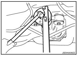
11. Remove companion flange using a puller.
