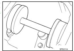
9. Select the correct standard pinion height adjusting washer thickness. Select by using a standard gauge of 3 mm (0.12 in) and your J-34309-101 feeler gauge. Measure the distance between the J-34309-11 pinion height adapter including the standard gauge and the arbor.
