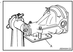
6. For proper reinstallation, paint matching marks on one side of the bearing cap.
