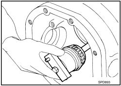
4. Assemble the pinion front bearing inner race and the J-34309-2 gauge anvil. Assemble them together with the J-34309-1 gauge screw in gear carrier. Make sure that the pinion height gauge plate, J-34309-16, turns a full 360 degrees. Tighten the two sections together by hand.
