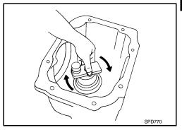
6. Measure the turning torque at the end of the J-34309-2 gauge anvil using preload gauge [SST: ST3127S000 (J-25765-A)].
