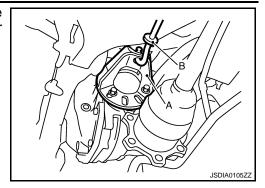
8. Measure the total preload with the preload gauge (A) [SST: ST3127S000 (J-25765-A)].
