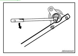
3. Put matching mark (B) on the end of drive pinion. The matching mark should be in line with the matching mark (A) on companion flange (1).
