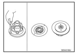
15. Separate differential case A and B, then remove viscous coupling, pinion mate gear, pinion mate thrust washer, side gear, pinion mate shaft, circular clip and side gear thrust washer from differential cases.
