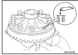
10. Install drive gear on the mounting bolts.
