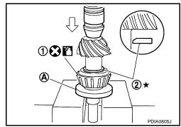
4. Assemble collapsible spacer to drive pinion.
