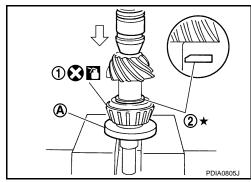
Assemble collapsible spacer to drive pinion. CAUTION:
