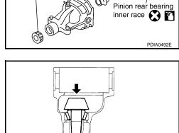
8. Using the drift (A) [SST: ST30720000 (J-25405)], install front oil seal as shown in figure.
