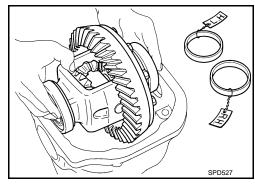
9. Remove side bearing inner race.
