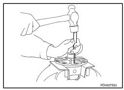
14. Remove pinion mate shaft.
